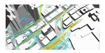
Wind From South-West direction passing through massing, directing wind through the center of the building
